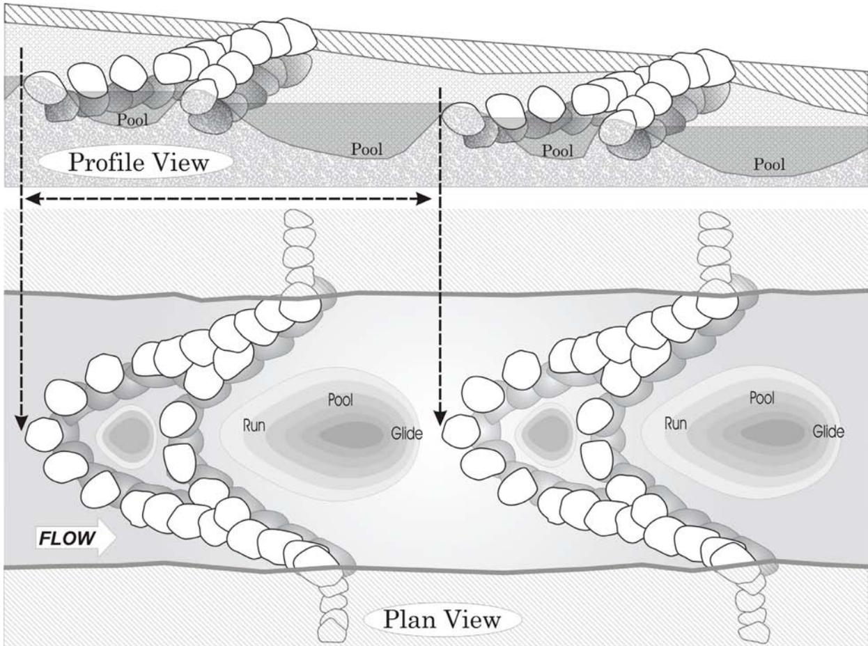
Figure 14. Use of Cross-Vane for step-pool restoration.
