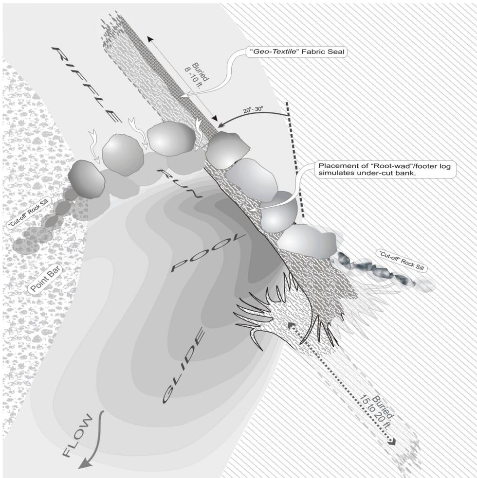
Figure 7. Root wad/log-vane/J-Hook combo streambank stabilization and fish habitat structure.
