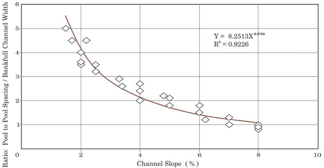
Figure 15. Ratio of pool spacing to bankfull width as a function of channel slope.
