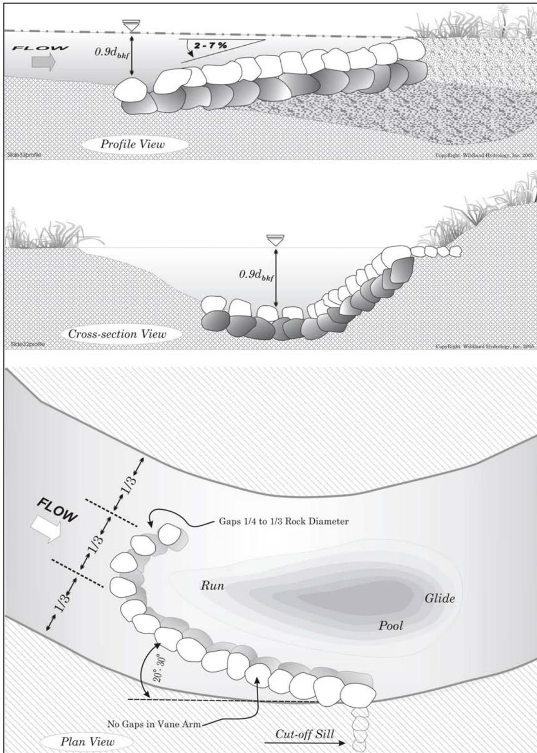
Figure 6. Plan, Profile, and section view of the J-Hook vane.
