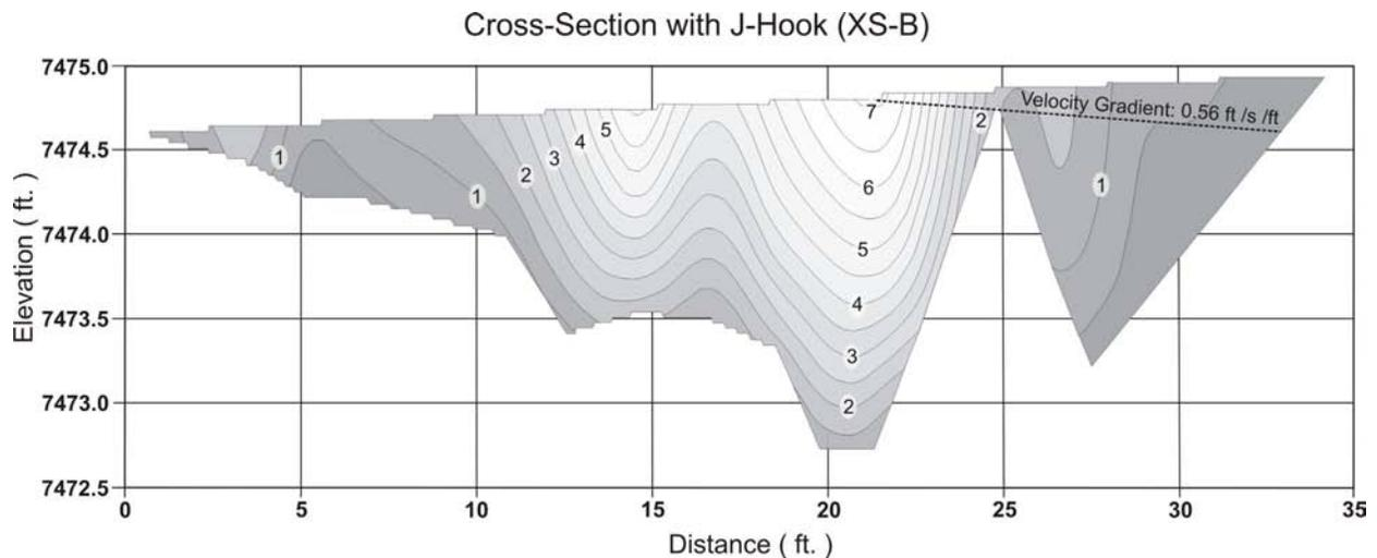
Figure 12. Velocity isovels of a J-Hook Vane, at Turkey Creek, Colorado. (Velocity in Ft./Sec.)
