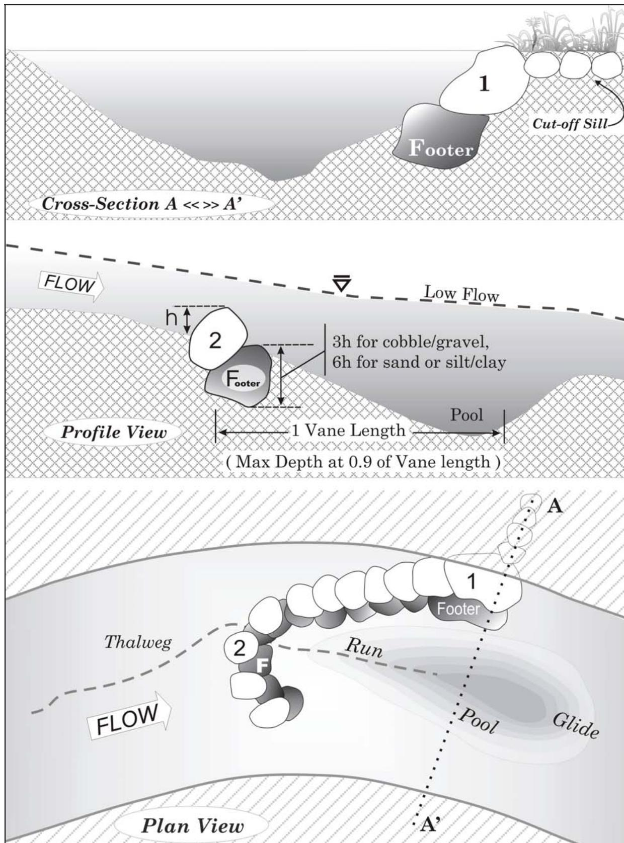
Figure 9. Locations – positions of rocks and footers in relation to channel shape and depths.
